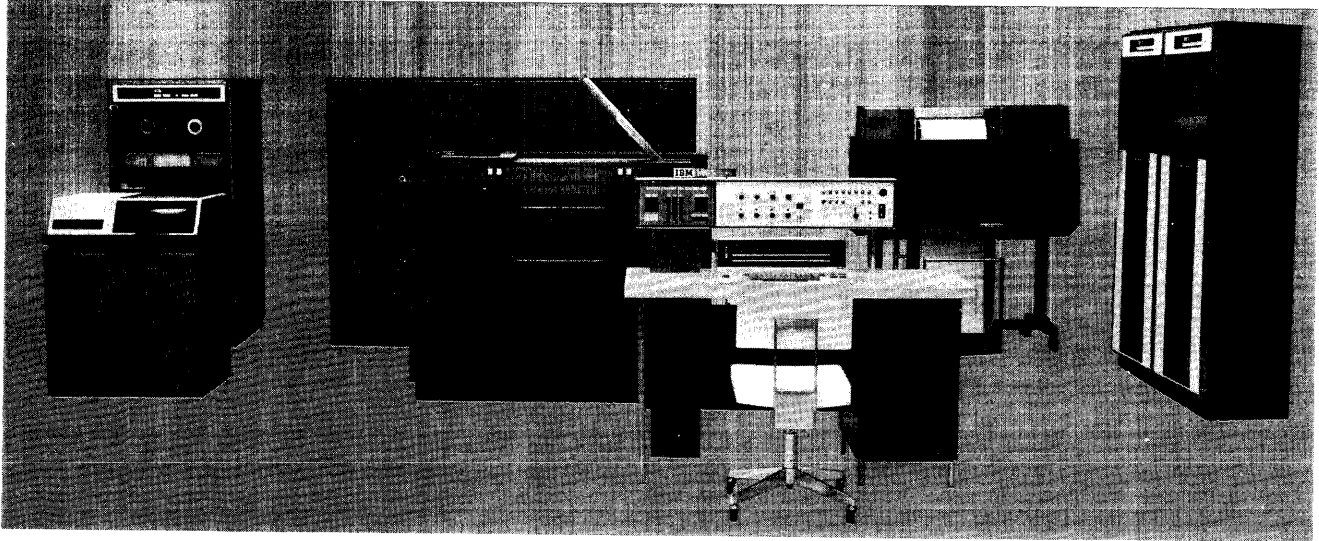
Figure 1. IBM 1460 Data Processing System
